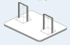
3. Device positioning is done via X&Y coordinates. For example, the installation direction of the master device is shown as below, the logo needs to be facing the front. When the master device's coordinate is (0, 0), the coordinates of the node devices are all positive values.
