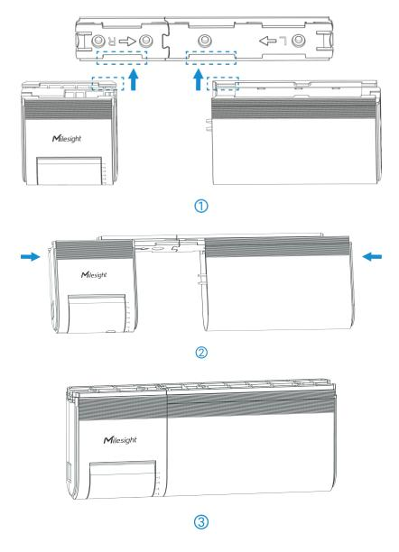
**Step 5:** Slide the two decorated plates to the side of the device.
