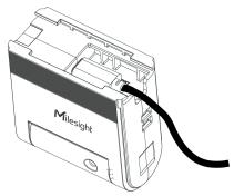
**Step 5:** Fix the device and the battery compartment to the mounting plate.
