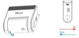
• Lintel Mounted: rotate the probe and make sensors straight face to the ground with the logo side.
