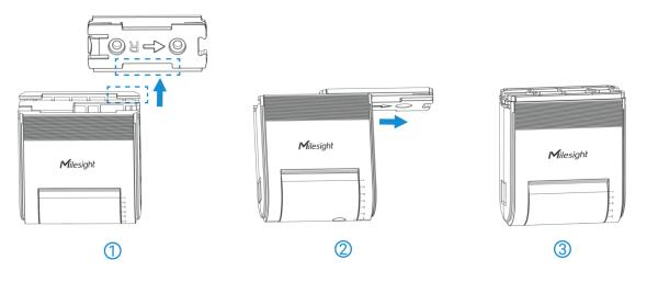
**Step 6:** Slide the two decorated plates to the side of the device.
