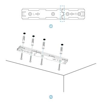
**Step 3:** Adjust the probe and installation direction.
